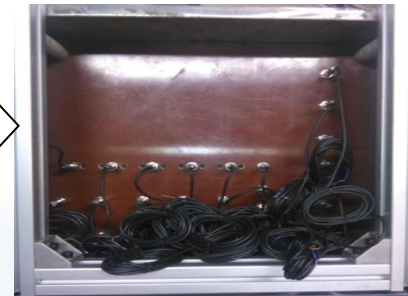
Bottom View of Gauge Table (Proximity Sensors to link Gauges and User Interface)
